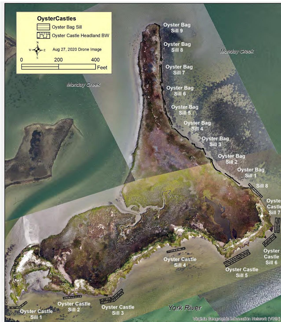
Figure 9. Proposed living shoreline project at Hog Island using oyster castles and oyster bags to create living sills along the shoreline for habitat restoration and shoreline protection.
